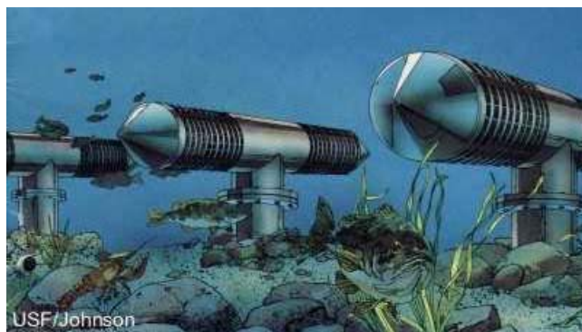
Figure 2-3: Drawing of Wedgewire Screens on the Bottom of a Water Body (Ref. (Ref. 7.4))
