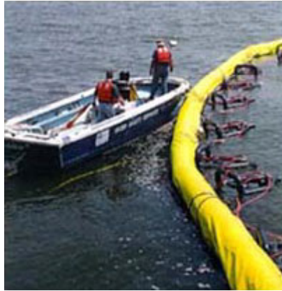
Figure 3-5: Deployment of the Gunderboom® Automatic AirBurst™ Cleaning System ( www.gunderboom.com )
